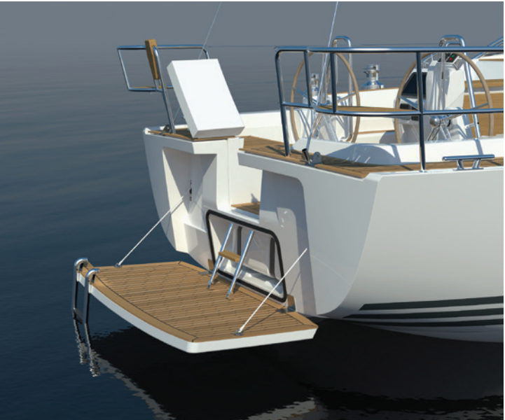
The large bathing platform is operated by a purchase block system. Below deck storage for a liferaft is accessed from the bathing platform.
