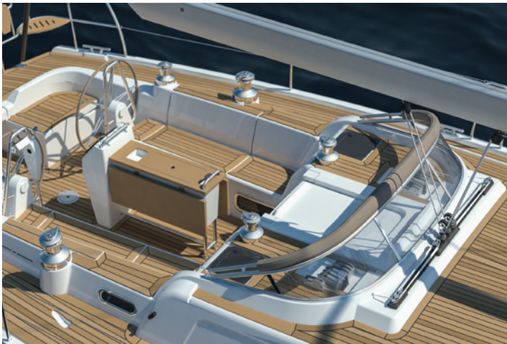
Xc 45 comes optional with an aluminium framed windshield with toughened glass.
