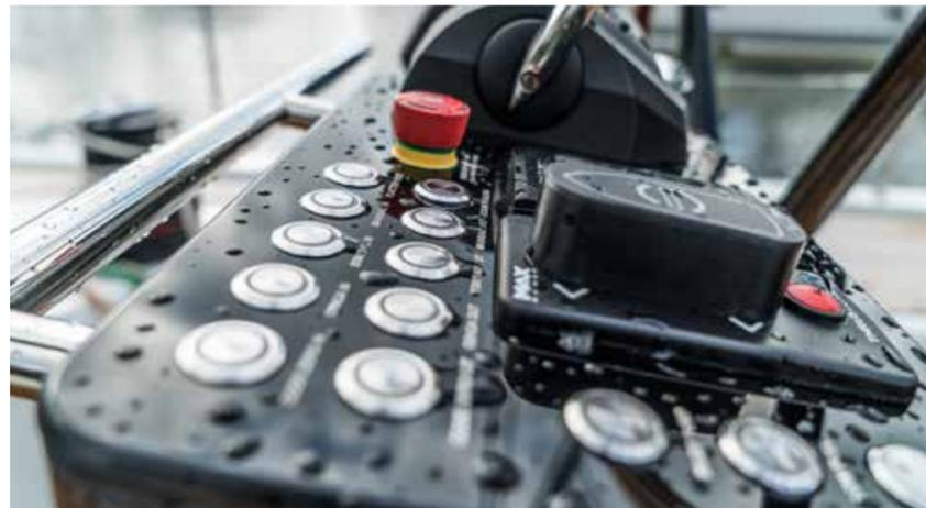
and instrument boxes to create a modern finish. All furling systems and engine controls are controlled from the push buttons on the console for easy short handed sailing.
