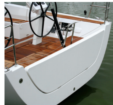
The optional folding transom creates a swim platform with telescopic swim ladder
