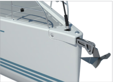
Standard GRP cowl with integrated anchor fitting
