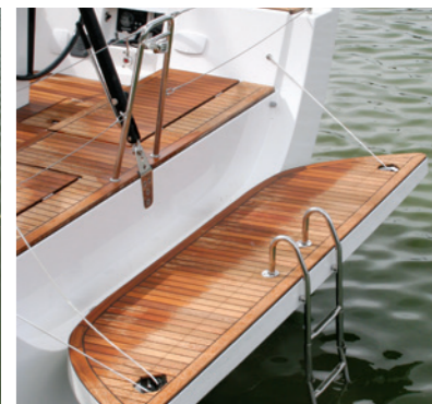
The optional folding transom creates a swim platform with telescopic swim ladder
