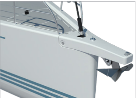
Optional white painted carbon bowsprit with integrated anchor fitting
