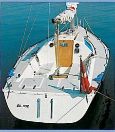
The cockpit is worked out providing optimum seating comfort at the 2 m long benches as well as on the side decks. The long mainsail cross haul secures a precise and easily operated mainsail trim. All halyards and reefs are led to the winch at the hatch garage so that it can be operated either from windward, leeward, or standing on the double step in the campanion way.
