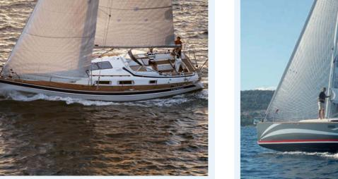
and is wider, shallower and flatter than the centre-cockpit 37's hull. Her mast is also taller and her keel slightly deeper and lighter. Flush hatches and below deck furler and windlass keep decks clear.
