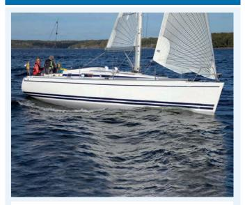
Arcona's sporty 370 is designed to be sailed by a small crew and, as with the X-Yachts, has an integral steel hull frame to which all the rig loads are taken and dissipated.
