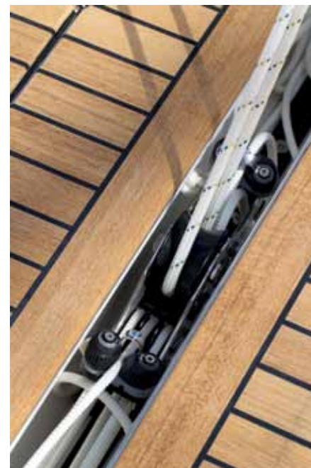
Above: The Xp 44 has a recessed mainsheet track giving a clean cockpit sole.
