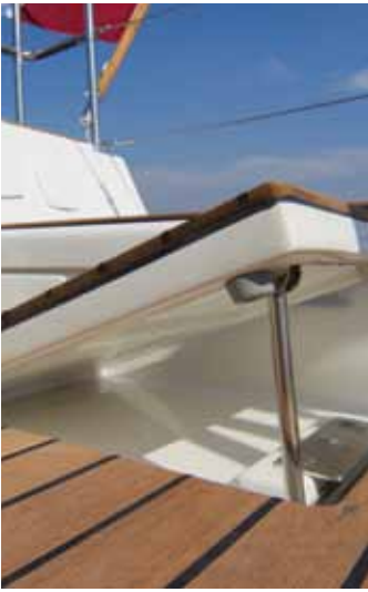
Above: Optional white painted carbon bowsprit neatly hides the standard removable anchor fitting.
