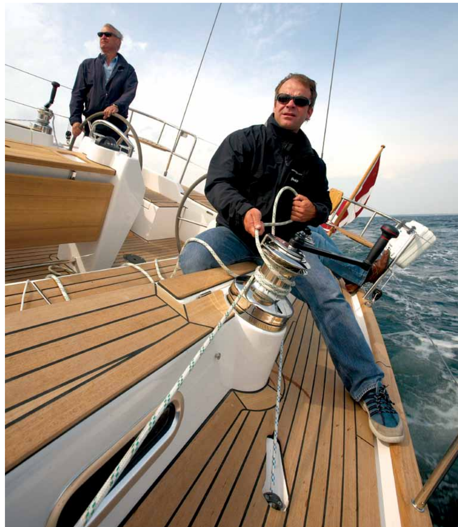
Above: Andersen full stainless self-tailing winches are standard equipment on the Xc 45.
