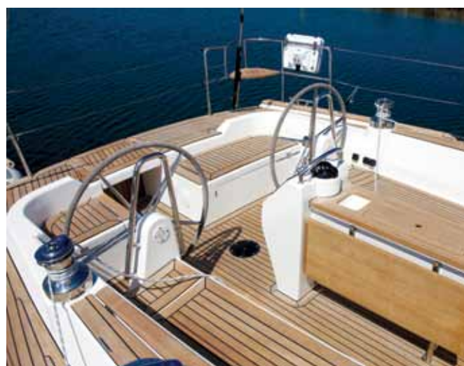
Above: The Xc 50 has twin wheels and a spacious cockpit area with a hydraulic folding transom that incorporates a bathing platform, plus liferaft compartment and additional storage.
