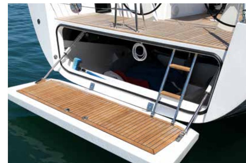
The transom tender garage includes an electrically operated door to form a convenient bathing platform
