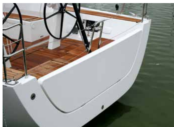
The Xp 44 features a folding transom with telescopic swim ladder
