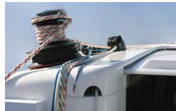
Jib control line under deck into cockpit
