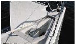
The recessed anchor box with electrical anchor windlass for cruising.
