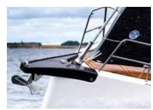
**Above:** The optional carbon bowsprit keeps the anchor clear of the vertical stem
