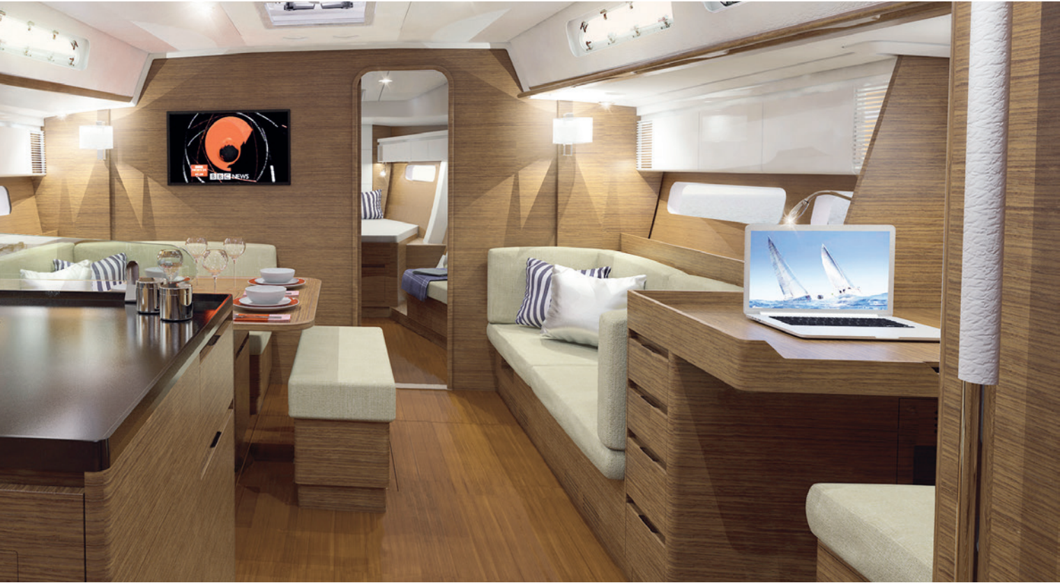
Above: optional interior surface options: Optional white top cupboards, veneered freeboards / lower cupboards in saloon, galley / nav station and owner's cabin. Optional black Corian galley worktop. Optional laminate floorboard in teak and holly.
