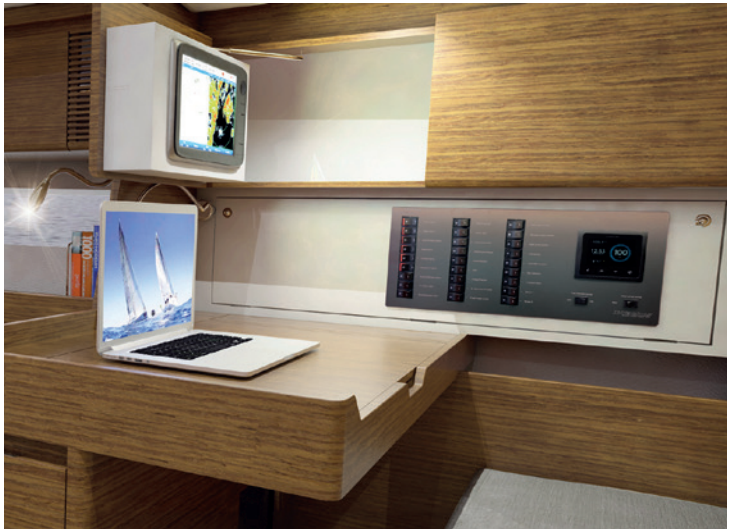
Above: The dedicated forward nav station with the chart plotter neatly hidden away in the top cupboard.
