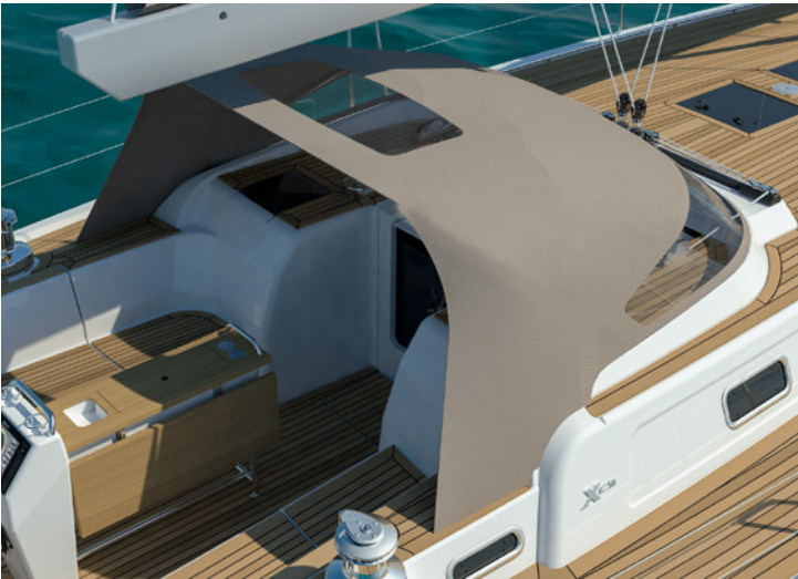
The standard spray hood is supported by three stainless steel frames. For canvas colour options, see pages 22-23.
