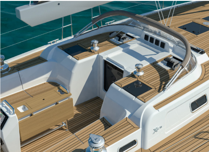
Xc 50 comes optional with an aluminium framed windshield with toughened glass.
