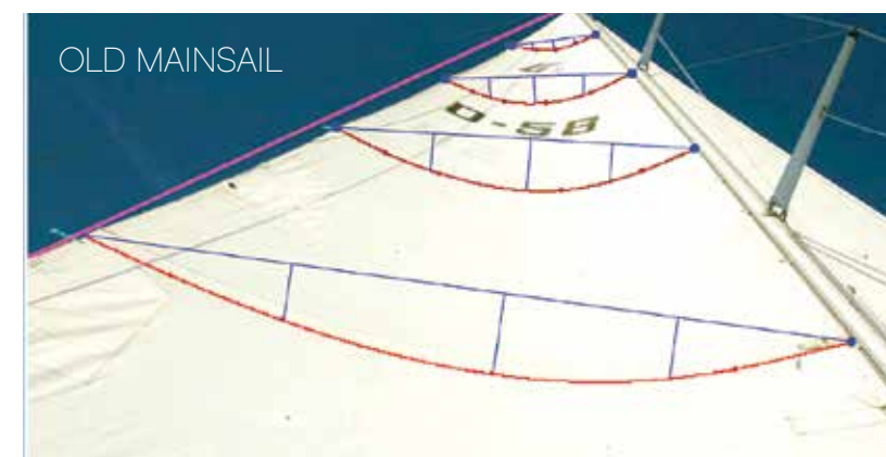
The old mainsail is first and foremost too deep, hollow, because the cloth is stretching, but it still twists OK at the top.
