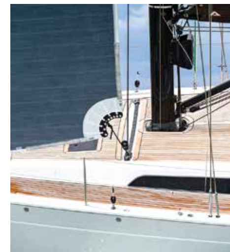
Different attachment points on the clew allow for subtle adjustment to jib twist when beating
