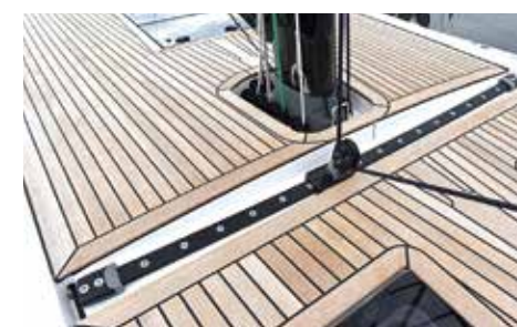
A self-tacking jib on an X? It helps make a powerful boat easy to handle when shorthanded
