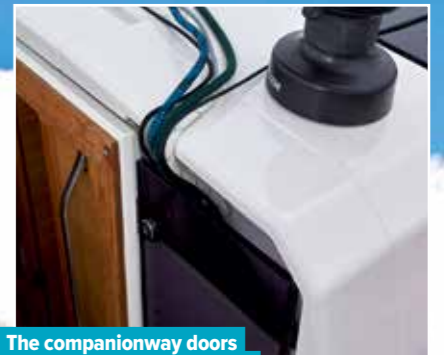
The companionway doors open into recesses that make up rope lockers for the coachroof lines
