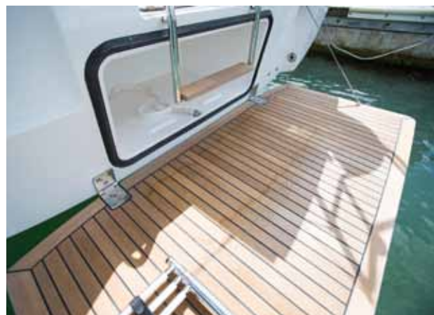
▲ Above: the swim platform is now twice the size, but the liferaft cannot be launched as easily. ▼ Below: secure side decks
