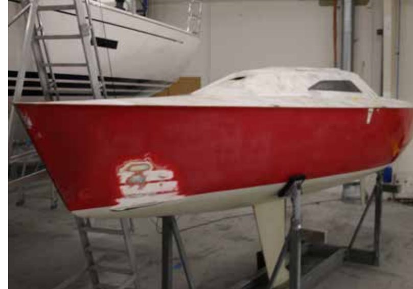
Sanding to find out whether the original water lines were still on the boat
