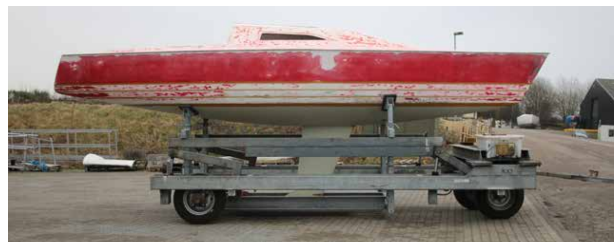
Deck after sanding. All holes closed and now ready for spray painting.
