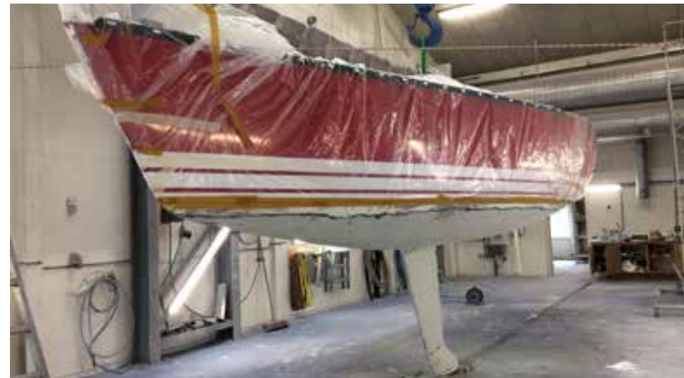
The boat has been spray painted and prepared for bottom primer and painting
