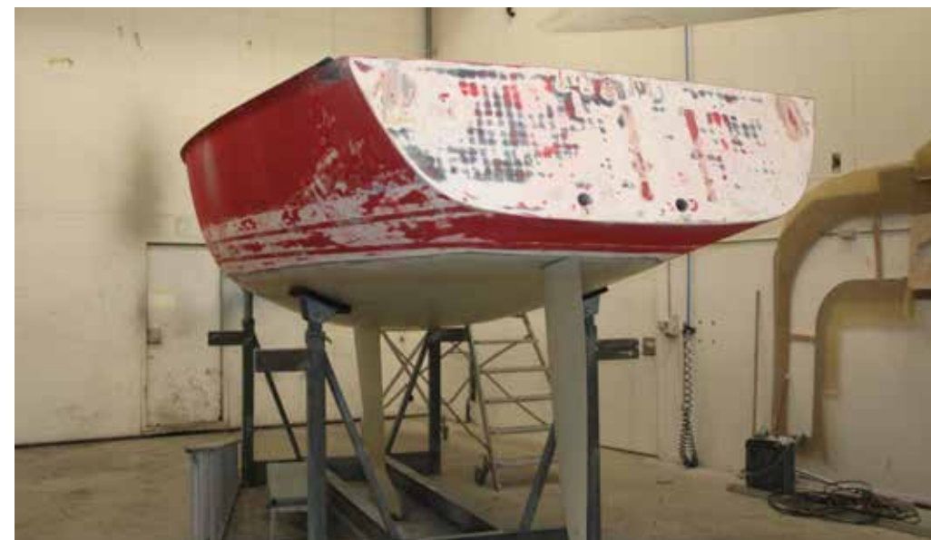
The hull after a full sanding and ready for spray painting
