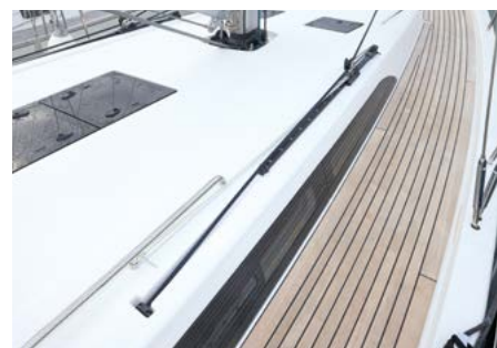
The genoa sheets and genoa car control lines are both led aft under the coachroof
