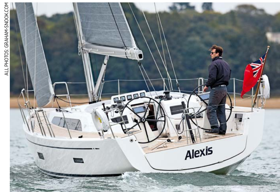
Fold-up footblocks make it more comfortable to steer standing up, and also allow you to brace your feet when sitting down
