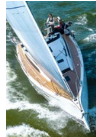
ABOVE: Narrow sheeting angles and a good set of sails let you point above 30° to the apparent wind, though best speed is just below that
