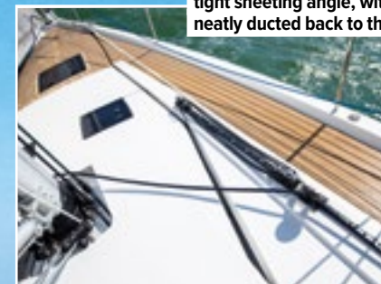
Chainplates are neatly hidden within the moulded toerails, and stanchions are neatly fitted
