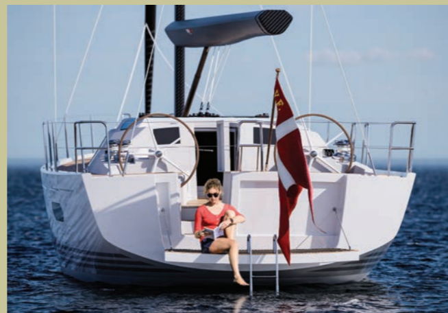
The aft end of the cockpit is enclosed and the transom folds down from an aft deck that serves as a helm seat
