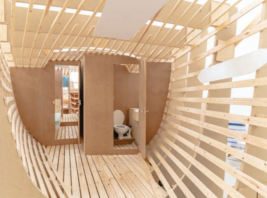
To check the ergonomics of the new Xc47 a full scale, heeling mock-up was built
