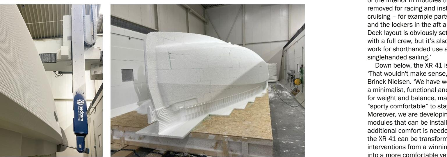
The XR 41 hull plug is being CNC machined with high precision and expertise at Nedcam in Holland
