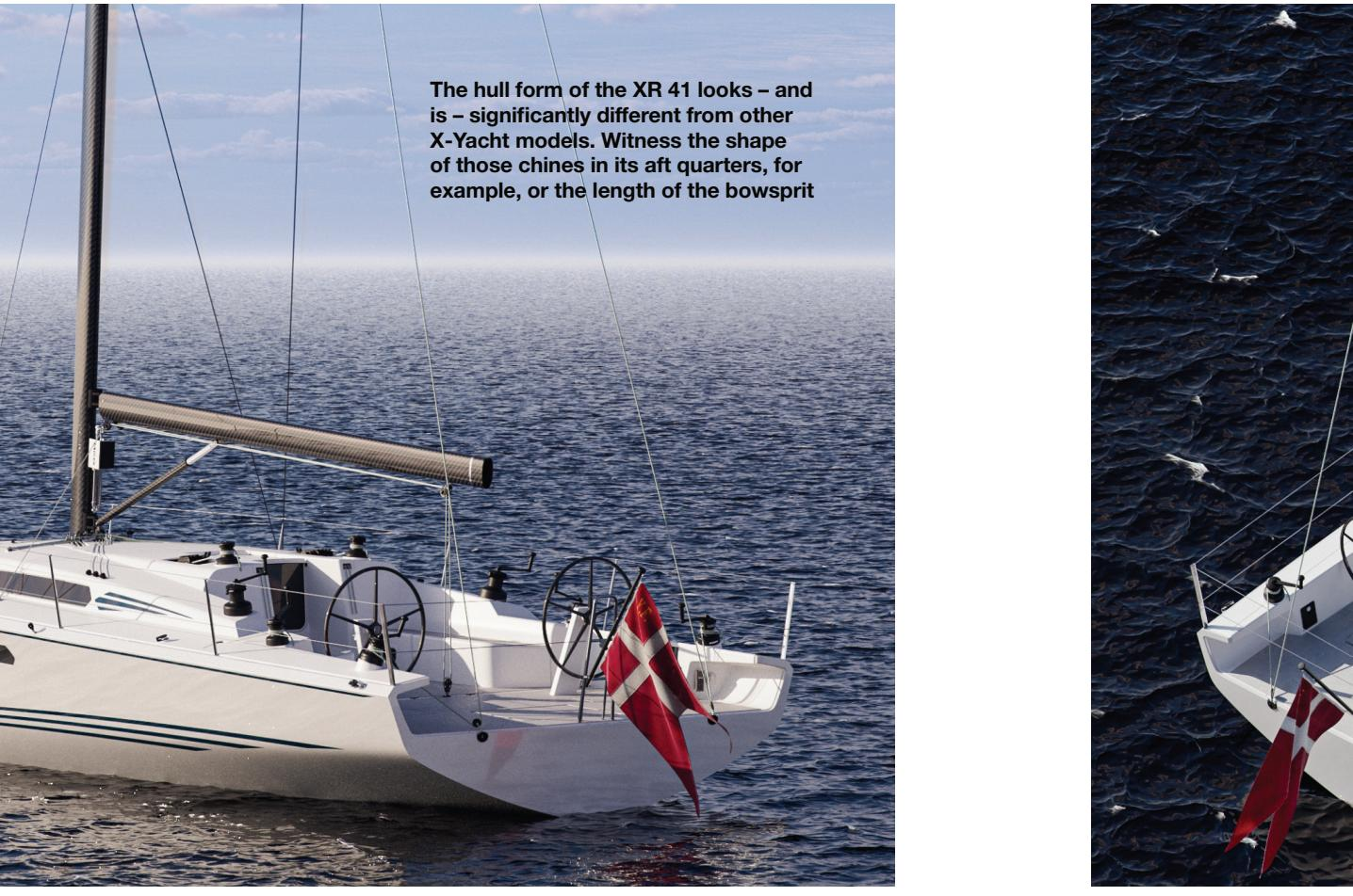
The hull form of the XR 41 looks – and is – significantly different from other X-Yacht models. Witness the shape of those chines in its aft quarters, for example, or the length of the bowsprit
