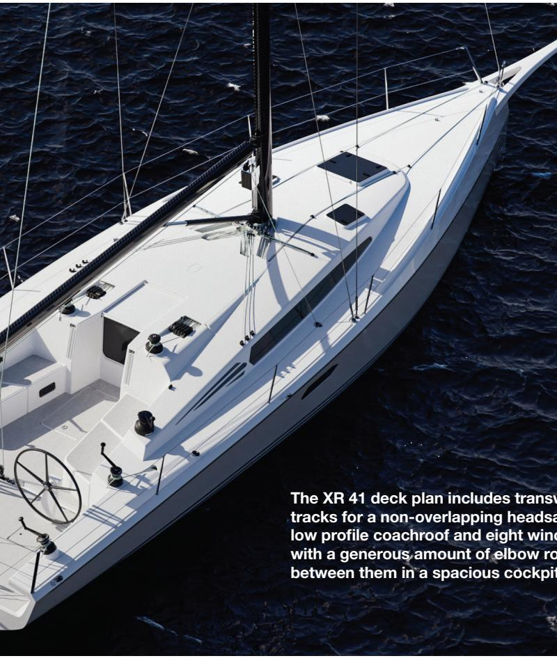
The XR 41 deck plan includes transverse tracks for a non-overlapping headsail, a low profile coachroof and eight winches with a generous amount of elbow room between them in a spacious cockpit
